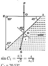
The angle of incidence at R continues to be  $45^{\circ}$  and since  $45^{\circ} < 70.53^{\circ}$ , refraction taking place and the refracted ray is RS. The angle of refraction r is given by  $\mu_g \sin i = \mu_w \sin r$
