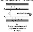
In a p-type semiconductor, the acceptor energy level  $E_A$  is above the top  $E_V$  of the valence band, therefore with a small supply of energy, the electrons can jump from the valence band to the acceptor energy level. Fermi levels shift closer to the valence bond because holes are the majority carriers. In a p-type semiconductor, the energy band increases.
